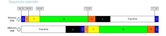
It is important to have the reset-time between shift changes. During this reset-time the control-unit is cleared, machine parameters are reset to original stage, and tools and tool holders are taken out. The machine is cleaned by the Competitor and made ready for the next shift to start their Test Project.
